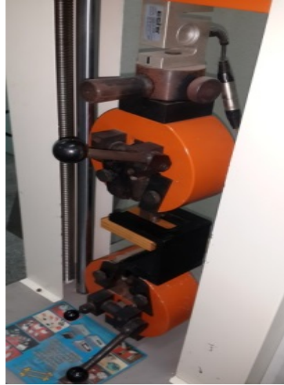
Fig. 4. Adhesion test machine and test sample.
