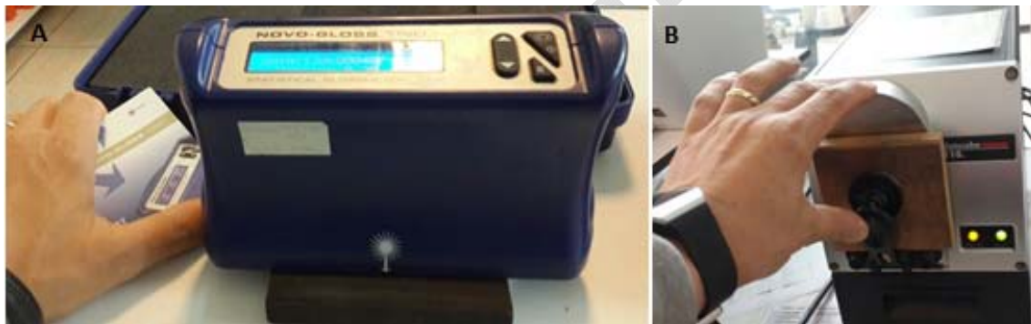
137 Fig. 2. a) Novo-gloss trio (60°) and b) The datacolor 110 spectrophotometer.
