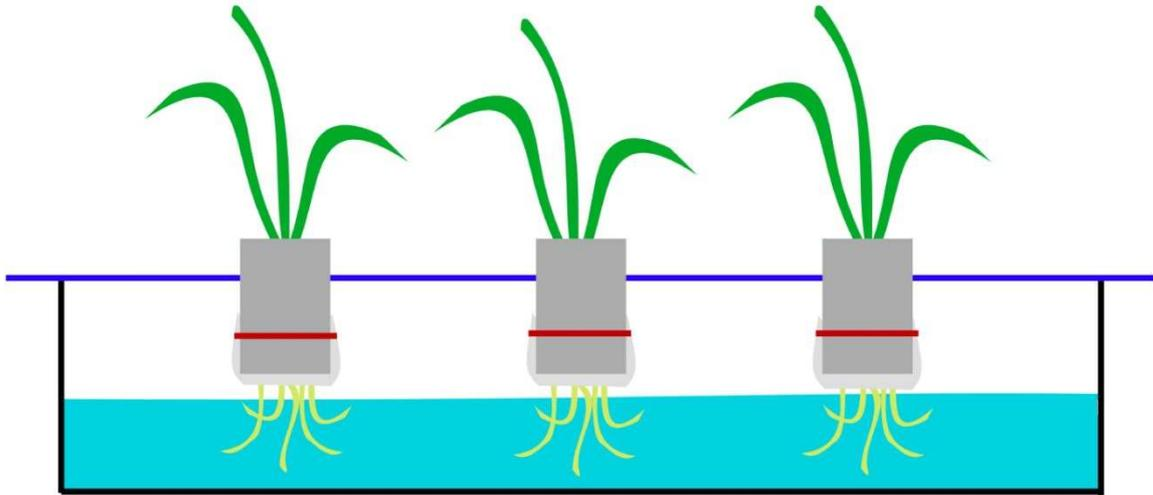
Figure 1: This is a schematic representation of the hydroponic system used for the experiment. It consists of a blue cover plate and a black painted box, both inhibiting photosynthesis and formation of chlorophyll in the leaves. Each plant is held in 5cm of an isolating tube fixed with cling film and an elastic band, so that the plant is fixed and the roots are in the nutrient solution. The solution is aerated in permanence to avoid any reactions varying concentration in the solution.
